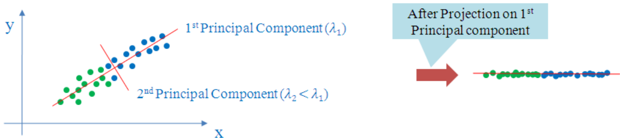
Figure 10 – Example of dimensionality (from D = 2 to d = 1 ) reduction using PCA
